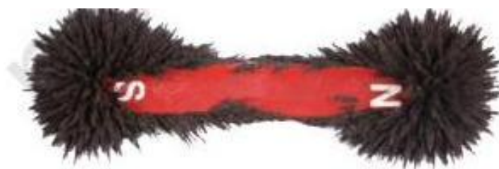
Fig. 4.4: Iron filings sticking to a bar magnet
