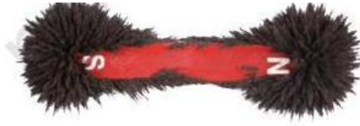
Fig. 4.4: Iron filings sticking to a bar magnet
