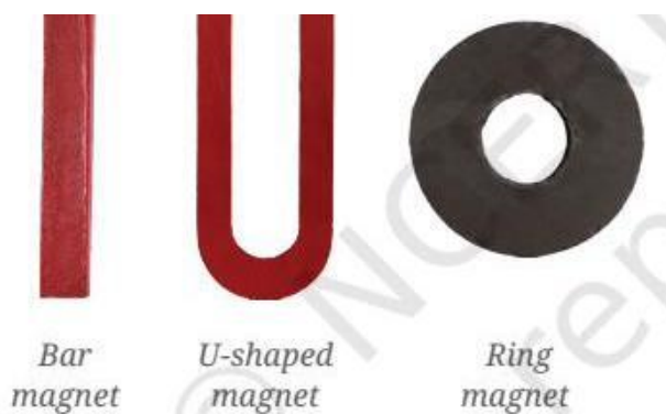
Fig. 4.2: Magnets of different shapes
