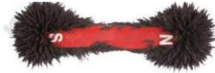
Fig. 4.4: Iron filings sticking to a bar magnet
